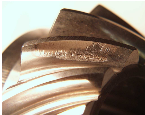
Figure 3 Pitting Damage on EX4
