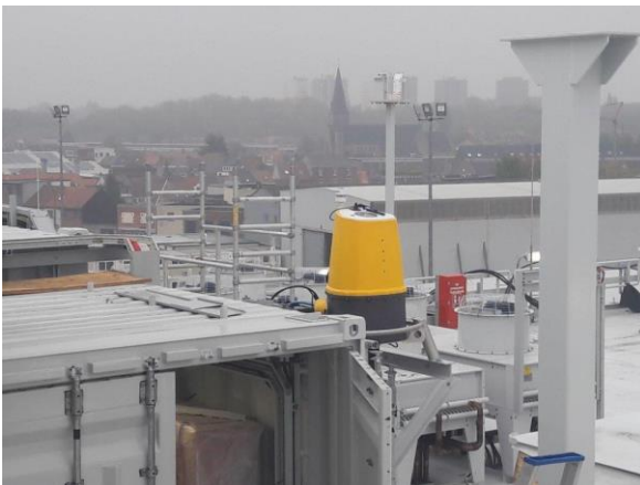
ZephIR 300M installed with ENGIE Fabricom during offshore substation fabrication.
