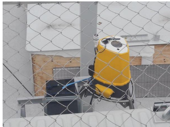
ZephIR 300M installed with ENGIE Fabricom during offshore substation fabrication.
