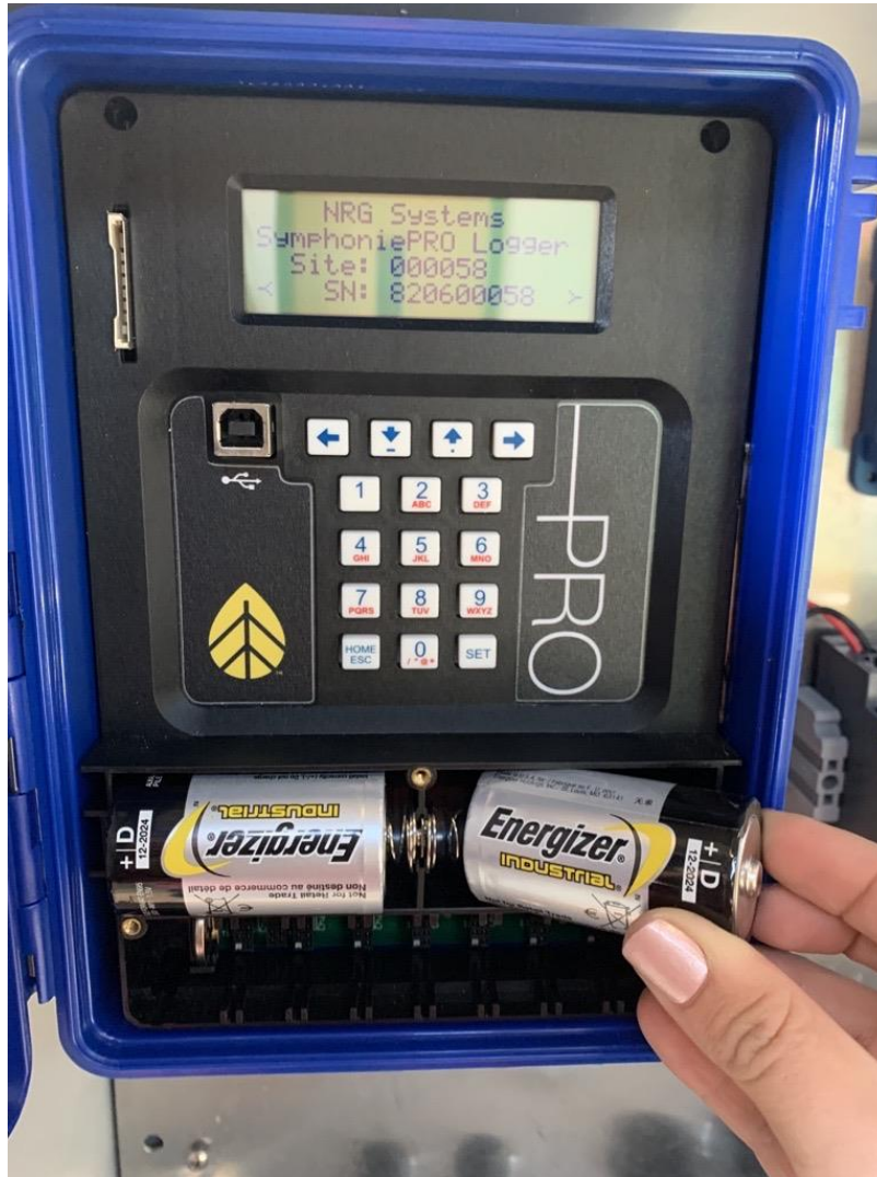
D-Cell battery insertion is shown above. The fabulous nails are not included.
