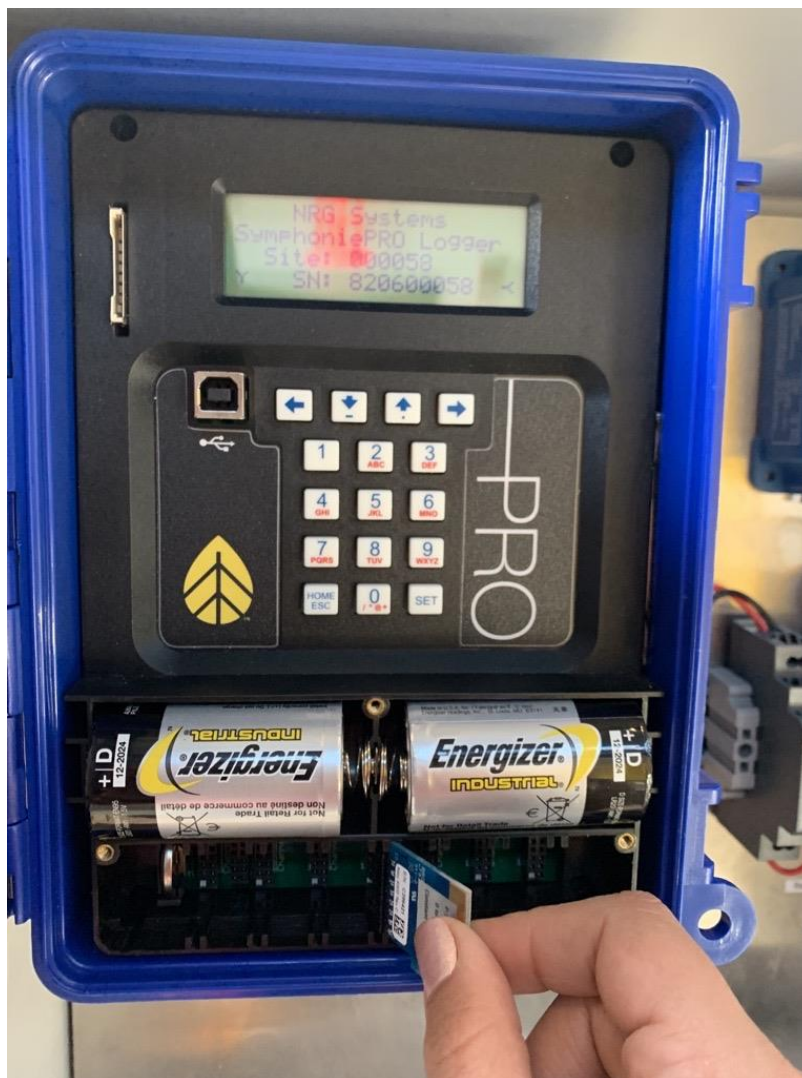
P-SCM cards are inserted below the D-cell batteries. Again, with the nails: gorgeous but unfortunately not included.
