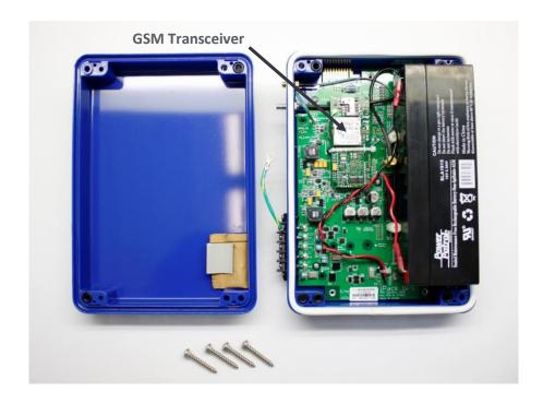
Newer GSM iPacks have the battery and electronics on the same half, as shown above. The GSM transceiver is located to the left of the battery.
