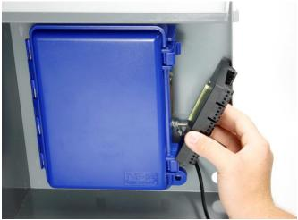
Note that the field wiring panel mounts over the grounding stud and can be removed from the logger without having to disconnect the sensor wires. This is particularly useful in the event a logger needs to be swapped out for service.
