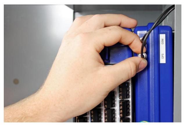
Satellite iPacks S/N: 35333300 and above have an SMA type antenna connector; older satellite iPacks have a TNC type antenna connector, so if you need to replace the older antenna or iPack, you will need an adapter.
