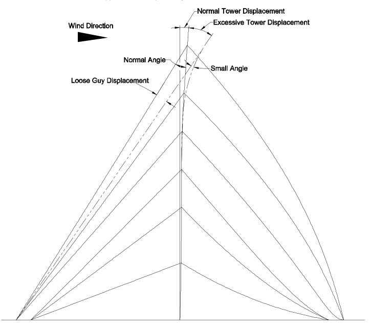
Picture 4-15: Snap-through diagram
