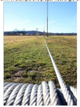
Picture 3-68: Correct winch cable fleet angle
