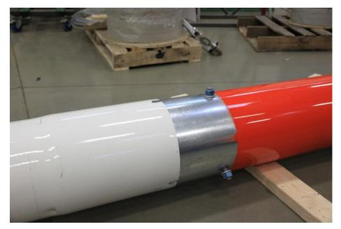
Picture 3-18: Sliding together tube sections
