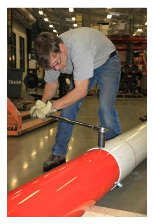
Picture 3-24: Torqueing the nuts
