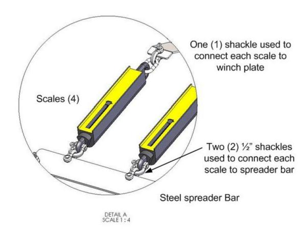
Picture E-2: Zoomed view of scale connection to winch plate and spreader bar
