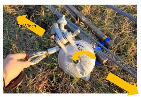
Picture 3-77: Reeving through pulley #5
