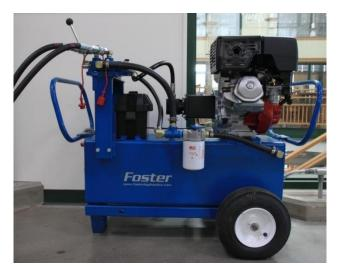
Picture 3-66: Foster Manufacturing Corp. HPU Model 13-1-8GC
