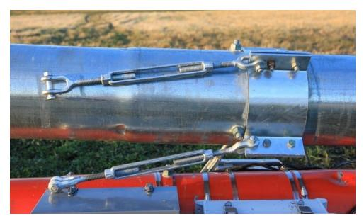
Picture 3-43: Turnbuckle assembly
