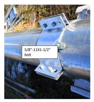
Picture 3-41: Ginpole jumper strut end-flange bolts
