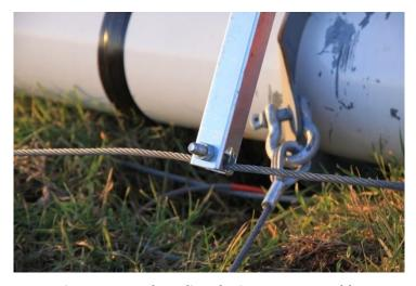
Picture 3-50: Threading the jumper strut cable
