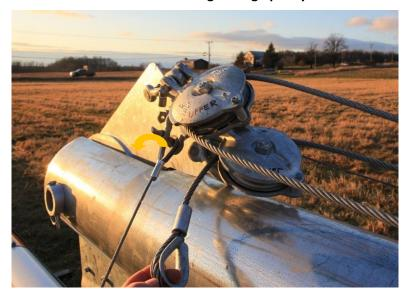
Picture 3-75: Reeving through pulley #4
