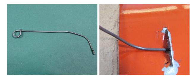
Picture 3-23: Example of tool that can be used to confirm tubes are mated together fully
