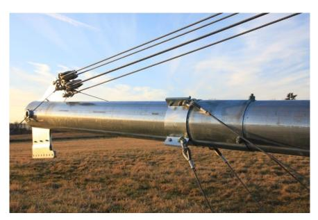
Picture 3-47: Jumper strut cable attachment
