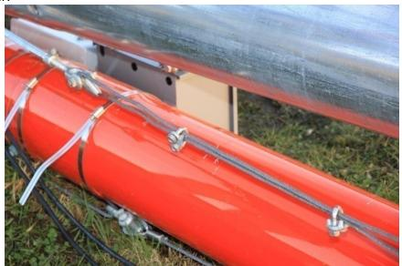
Picture 3-51: Attach jumper strut cable to turnbuckle
