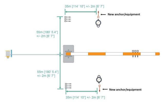
Picture 2-4: Layout drawing showing location of back stay tensioning system
