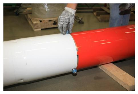
Picture 3-20: Nuts/bolts hand tightened
