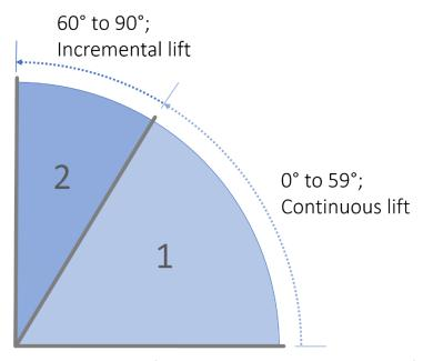
Picture E-5: Phases of the Super 60 & 80m XHD TallTower lift
