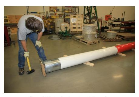
Picture 3-21: Seating the tubes with a mallet
