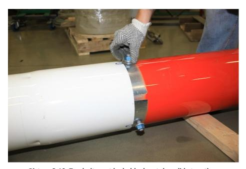
Picture 3-19: Top bolt must be held when tubes slide together
