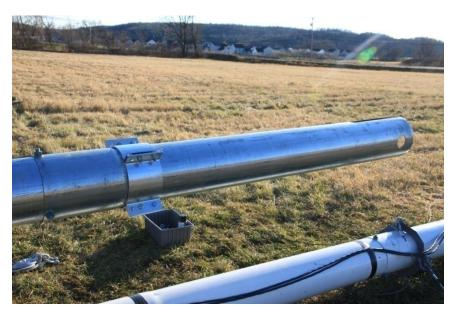
Picture 3-42: Ginpole jumper strut end-flange
