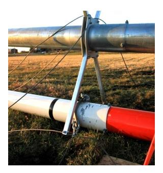
Picture 3-49: Threading the jumper strut cable
