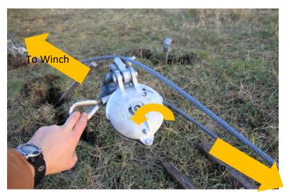
Picture 3-74: Reeving through pulley #3
