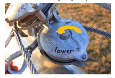
Picture 3-76: Reeving through pulley #4
