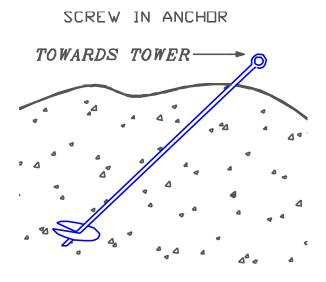
Picture B-1: Installing Screw-in Anchors
