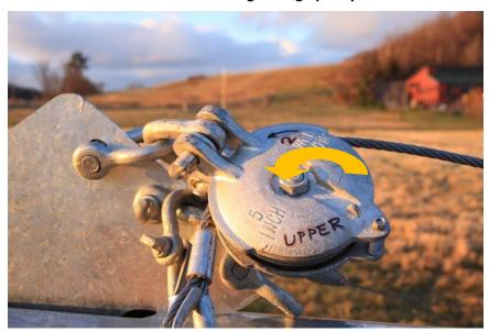
Picture 3-73: Reeving through pulley #2
