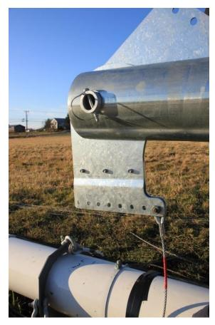
Picture 3-56: Lifter attachment to rocker plates
