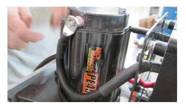
8. Once the leads are attached, the winch should be ready for use.
