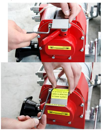
**Step 1:** Remove 2 Allen screws and the old safety mechanism as shown below.
