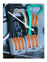
In a correct assembly, the connector block with the green wire, or yellow wire with the green stripe, should be connected to the lead on the diode that has the silver stripe around its body.
