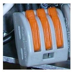
Shown above is an example of the type of connector block used in wiring type 2. It should be noted that all wires attached to a single connector block are essentially wired together.
