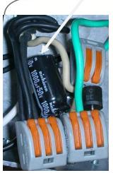
In a correct assembly, the connector block with the black wires will be connected to the capacitor lead on the side with the silver band.
