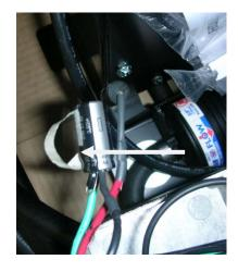
In a correct assembly, the lead on the side on the diode with the silver band will connect to the green wire.
