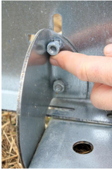
Figure 4: Attach the Gusset to the Vertical Baseplate
