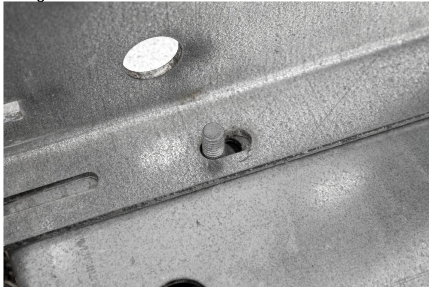
Figure 3: Attach Vertical Baseplates to Horizontal Baseplates
