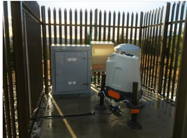
Figure 1: The simple, low-profile wind lidar ZephIR 300 now SCADA integrated in replacement of the Permanent Met Mast
