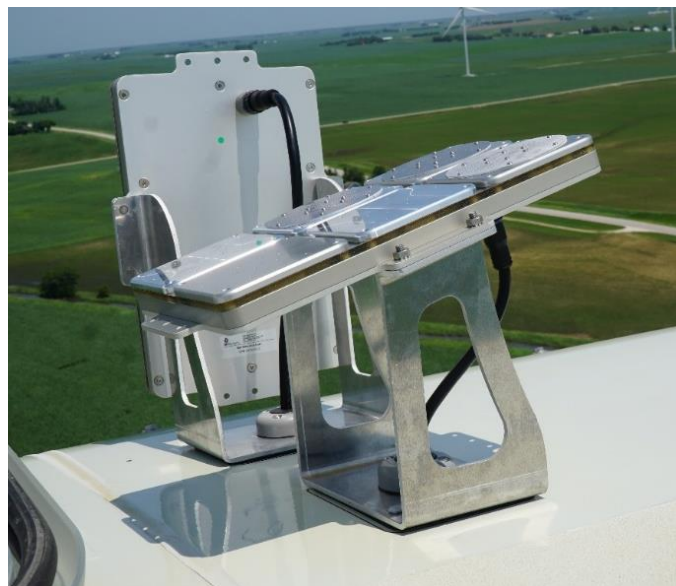
Bat Deterrent Units mounted on the nacelle of a wind turbine.
