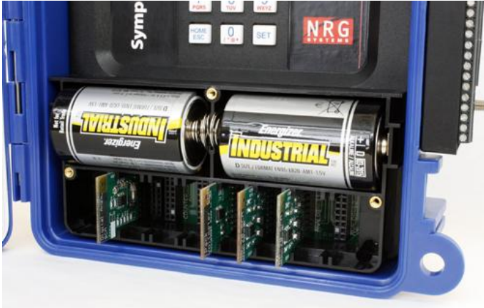
SCM cards installed under battery cover
