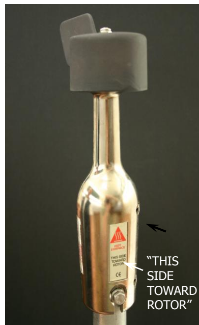
Slide sensor down over mast.
