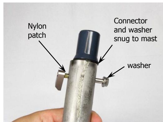
Secure connector to mast with bolt, washer, and nut.
