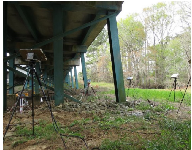
Figure 6. BDU Arrangement Around Expansion Joint
