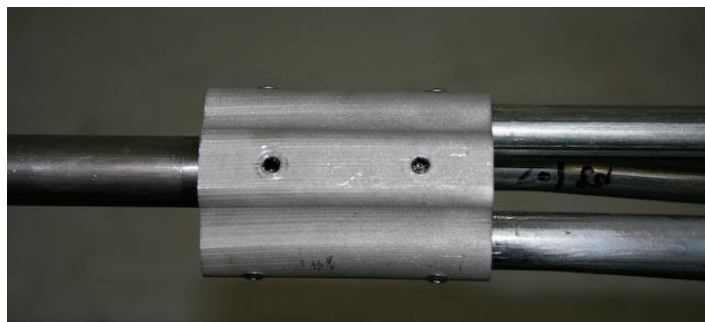
Figure 1 | Boom sleeve with holes visible
