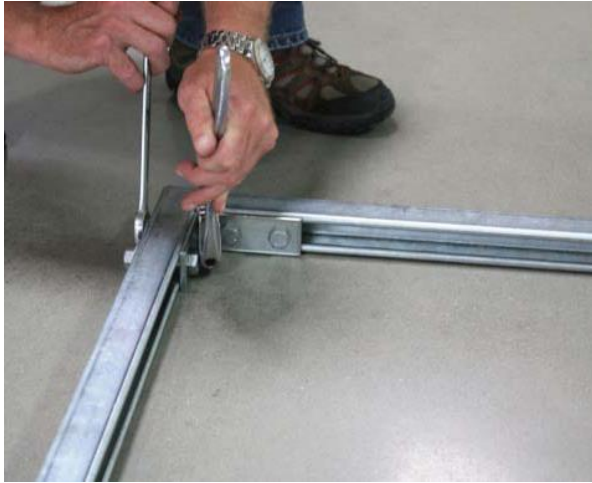
Figures 3 & 4 | Assembling the brackets & Completed brackets
